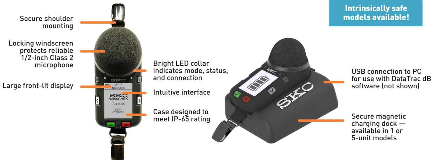
\*Use with intrinsically safe models may require an intrinsically safe mobile device.
