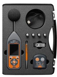
SoundCHEK sound level meters are supplied in a protective case with foam that accommodates the AcoustiCHEK Calibrator. (Calibrator sold separately - see ordering on p. 2).
